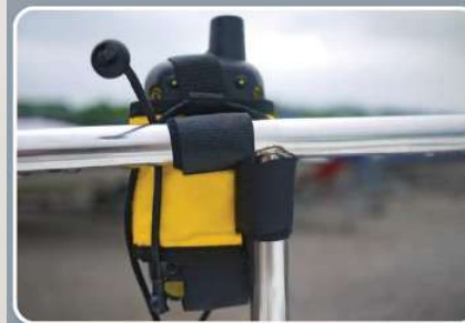
Examples of Good Mounting Positions
